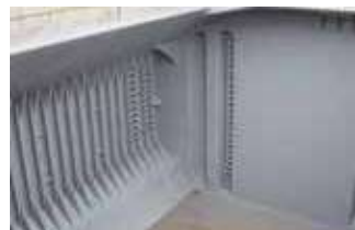
Abrasion resistance coating for Cargo Hold
