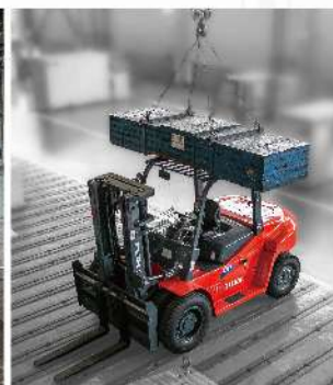
Impact test of overhead guard
