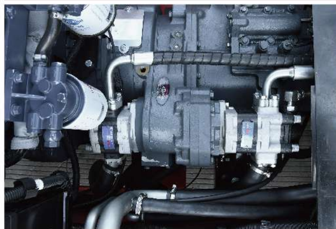
Load sensing steering and dual pump confluence technology, energy consumption reduce by 10%
