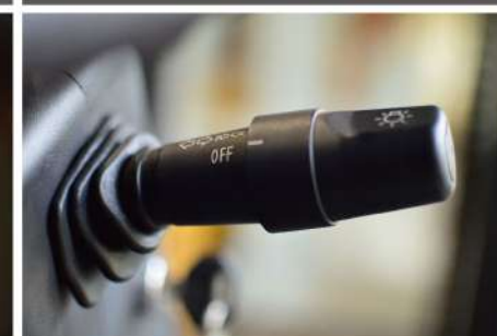
Integrated light switch
