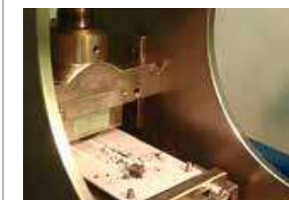
Coal scratch test
